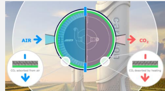
Carbyon's direct air capture process minimizing energy consumption
