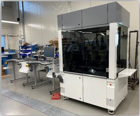
Automated manufacturing solutions. Example: Precision assembling station for IVD test cards
