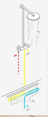
to the upstream heat exchanger. The waste energy of the used shower water pre-heats the incoming cold water, which reaches the mixing valve already warmed, so less hot water from the boiler is needed to enjoy a relaxing warm shower. The Joulia heat exchangers recover up to 63% of wasted heat.
